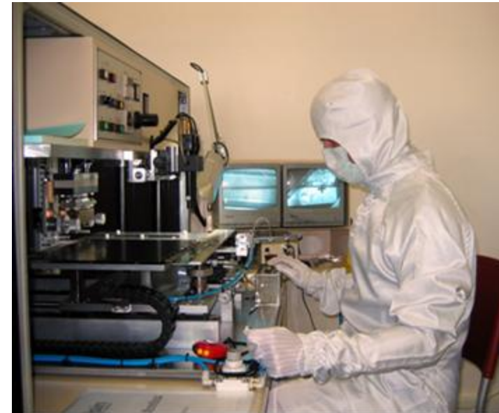
Bonding operation in ELSIN Ltd.
